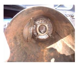
After cleaning, it was necessary to file the "serrated edge" effect of the cylinder to a smooth finish and generally tidy up the edges.
