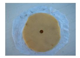
The replacement filter fits neatly into the front containing area (the AF cap), slides over "mushroom" of the centre spindle, is crimped slightly each side, and then slid home into the filter cylinder.
